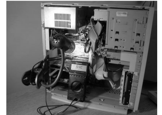
Figure 3. Experimental setup to induce memory errors, showing a PC built from surplus components, clip-on gooseneck lamp, 50-watt spotlight bulb, and digital thermometer. Not shown is the variable AC power supply for the lamp.
